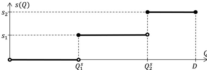
Figure 3. Step function of the discount  $s(Q)$  on stored inventory
