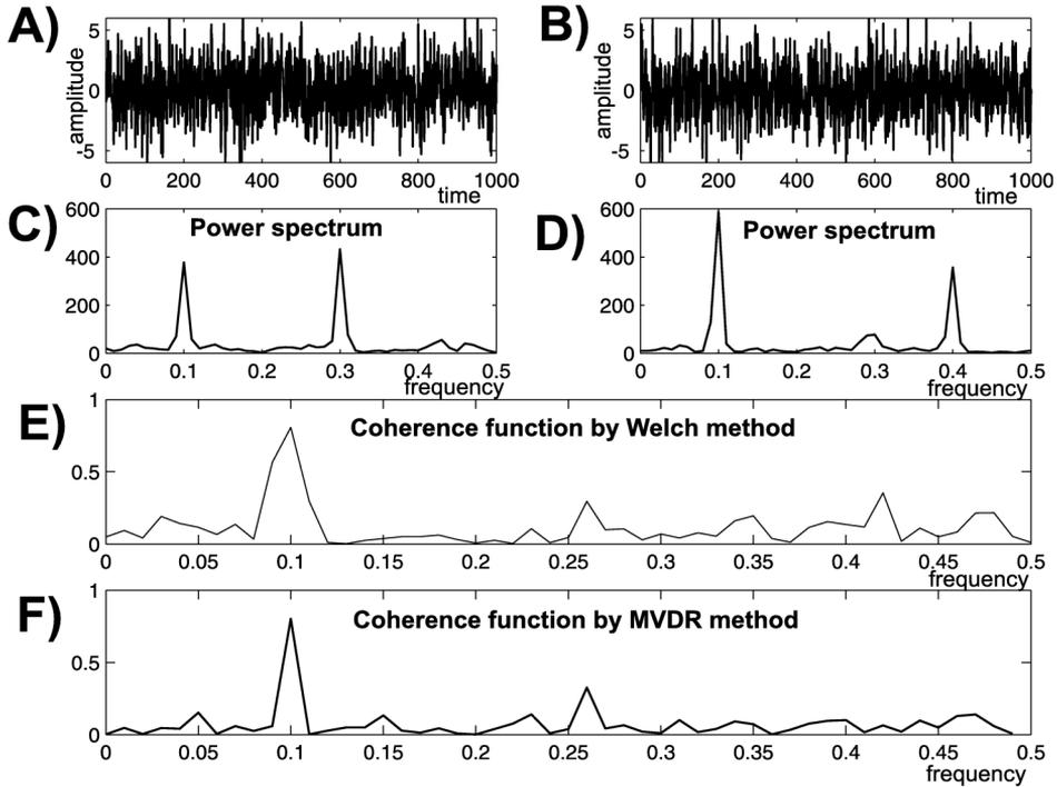
Fig. 1. Example of coherence function: A) signal  $x(n)$ , B) signal  $y(n)$ , C) power spectrum of signal  $x(n)$ , D) power spectrum of signal  $y(n)$ , E) coherence function by Welch method, F) coherence function by MVDR method (common frequency for two signals 0.1 Hz)
